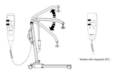
• On models with Integrated APC, push the seated person buttons on the hand control and confirm the cradle re-positions accordingly.
