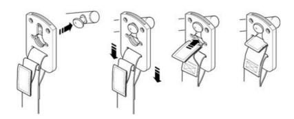
Securi3 sling attachment system. Example of installation.
