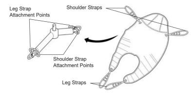
6-point spreader bar. Example of 6-point spreader bar sling with loop attachments.
